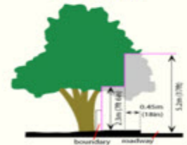
Trimming over footpath and roadway
