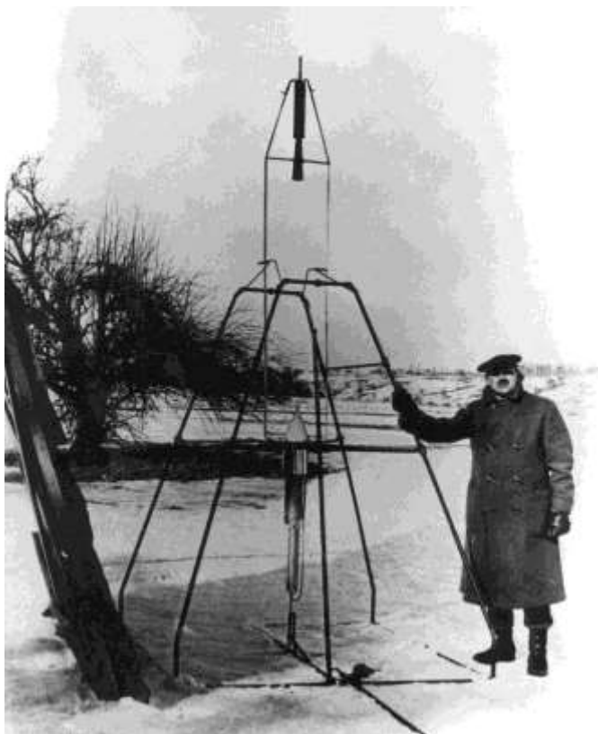
American Robert Goddard 1926. The rocket engine is at the top. The bottom is the fuel tank. Internet
