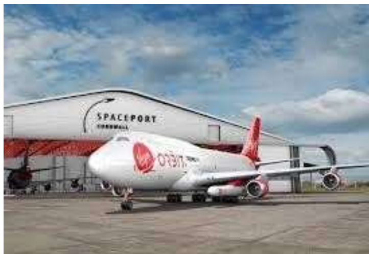
Spaceport Cornwall. Rockets carrying satellites are launched from beneath the 'plane which carries them to a high altitude first. Internet
