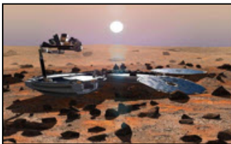
Beagle 2 as it should have deployed. One panel has not opened and traps the antennae.
